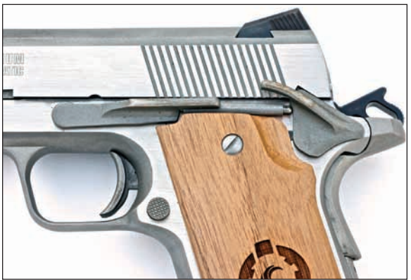
The left side controls are exactly like the M1911's. The grip safety's tang is extended and there is no possibility of bite from the Commander-style hammer.
