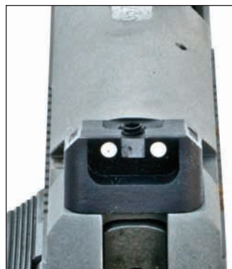
The Coonan's black, fixed tactical-type sights are excellent. The front blade has a single white dot. The open square-notch rear has a white dot on each side.
