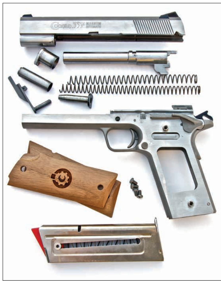
Disassembly procedures are precisely those of the M1911 Government Model pistol and present no problem to those familiar with the famous caliber .45 ACP series.
