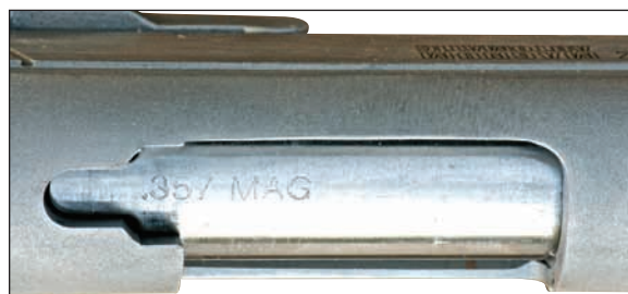
The large ejection port was specifically designed to accommodate the long, rimmed .357 Mag. case. The slide top has a bead-blasted finish to reduce glare.
